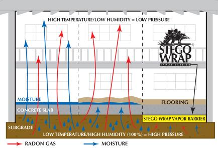
Regardless of the location of the water table, humidity below concrete slabs approximates 100%. Typical below slab vapor pressure is more than twice that of building interiors at room temperature, creating vapor drive from the substrate, up through the slab, and into the building.
